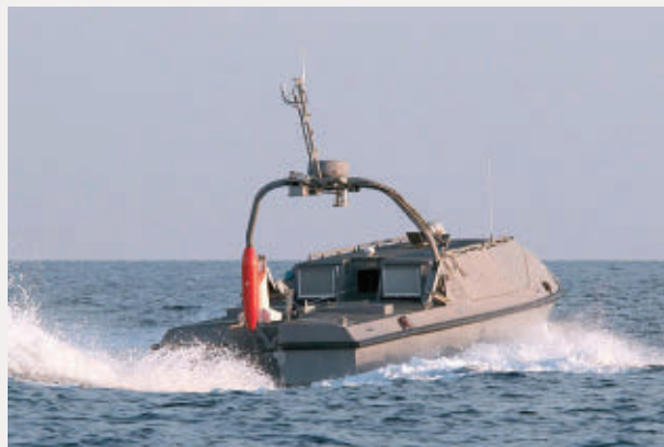
AAI is developing an unmanned boat for the Navy's Littoral Combat Ship that will help with mine warfare operations.
